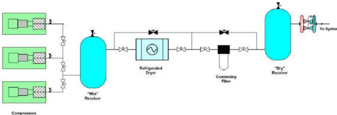
Let us assume three identical rotary compressors and a dryer and filter sized to match the total output of all three compressors. The “wet” receiver is the “control” receiver, while the “dry” receiver provides storage of dried and filtered air.
