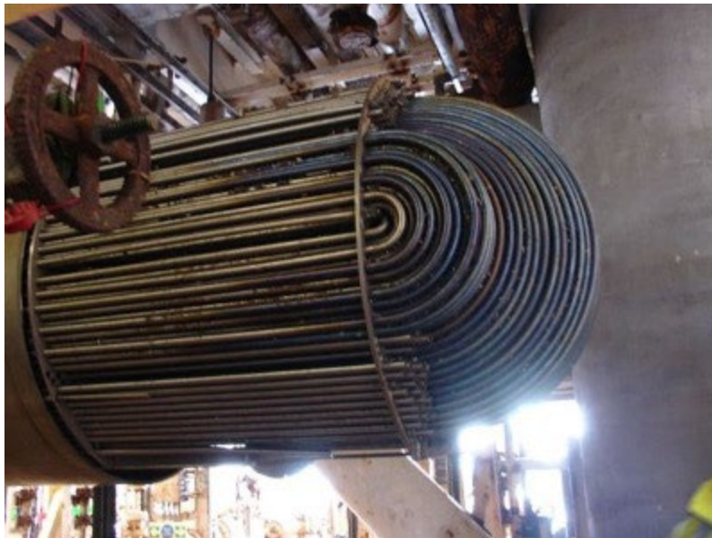
The tube bundle of a heat exchanger.
