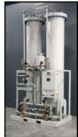
Mid-sized PSA N 2 generator as often used for laser cutting operations – produces 5700 SCFH of 99.99% N 2 (less than 100 ppm of O 2 .)
