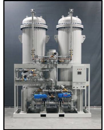
A large PSA style N 2 generator such as might be used for circuit soldering applications – capable of 10,500 SCFH of 99.995% N 2 (less than 50 ppm O 2 .)
