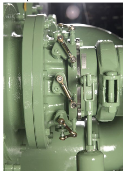
Figure 3: Side-view of mounted IGV showing the yoke assembly and actuator.
