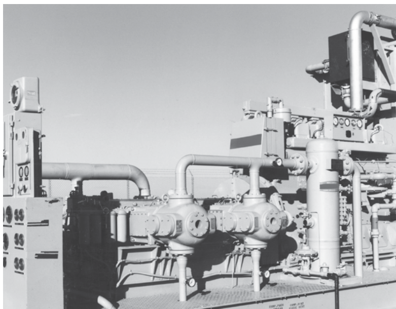
Figure 7.18 Field installation of a balanced opposed, two-stage compressor in gas lift service.
