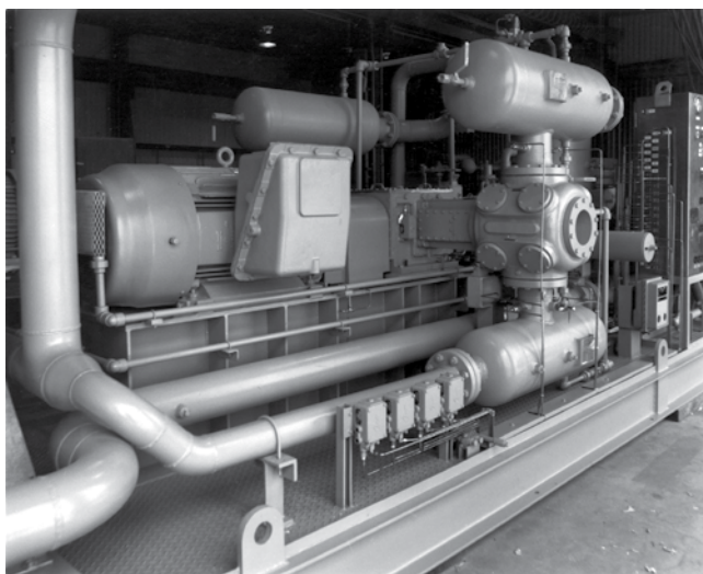
Figure 7.92 Induction Motor-driven Oil Field Compressor Package
