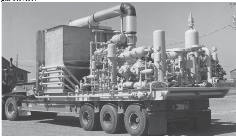
Figure 7.98 Field installation, 32 Bhp, 1400 rpm integral engine-compressor in casing-head gas service.
