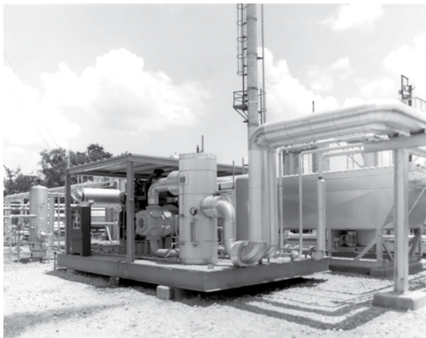
Figure 7.90 Gas engine-driven two-stage compressor in a mini-gas plant.
