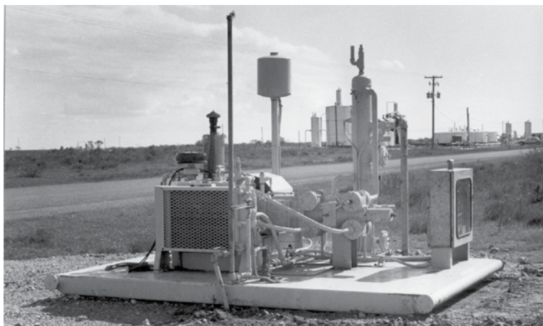
Figure 7.36 Two stage, 13 hp portable package compressing 60,000 cfd of flash gas from oil well separator into 400 psig gas gathering system.
