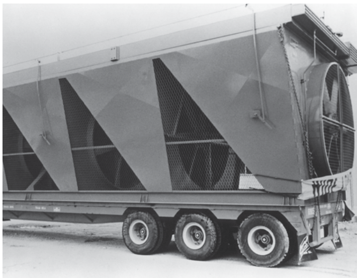
Figure 7.85 Air-cooled heat exchanger during transport to job site.
