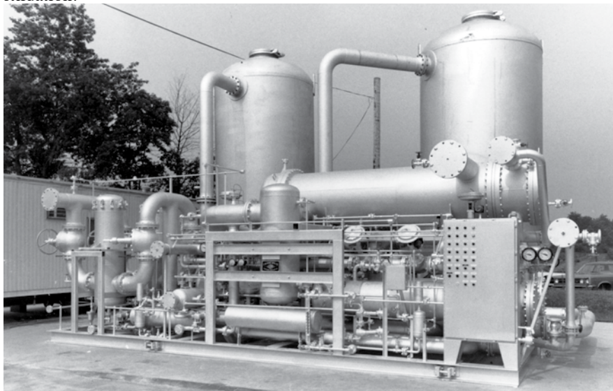
Figure 7.169 A carbon dioxide gas dryer operating at 720 psig for a chemical plant.
