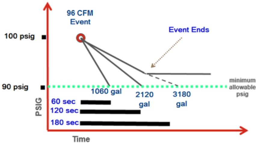
Figure 4.22 Effect of control storage on rate of change
