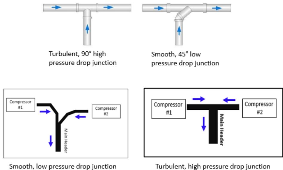
**Figure 4.14 Various piping transitions and their associated pressure drops**
