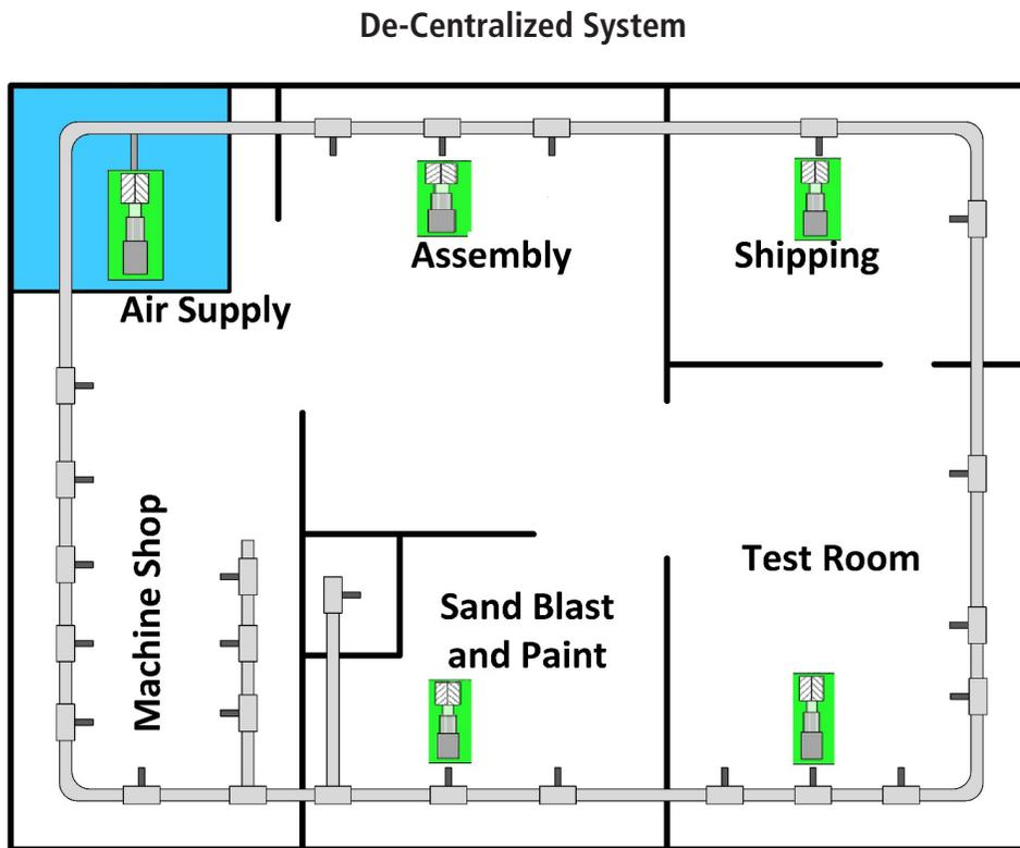
**Figure 4.16 De-Centralized layout**
