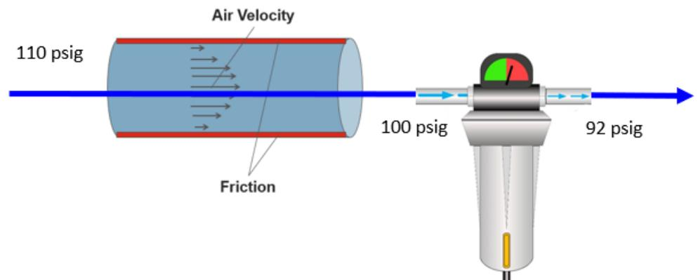
**Figure 4.1 Pressure drop as a function of friction due to resistance to flow.**
