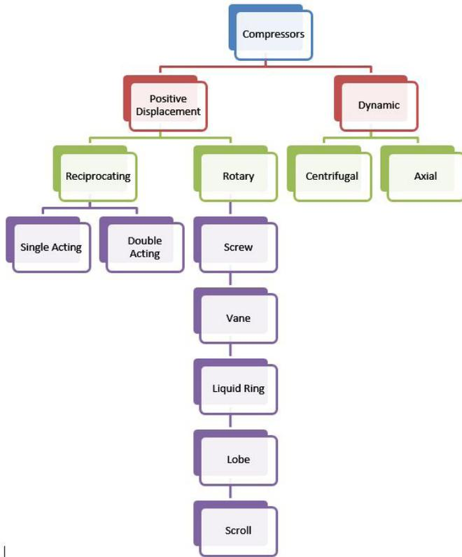
**Figure 4.9 Types of Compressors**
