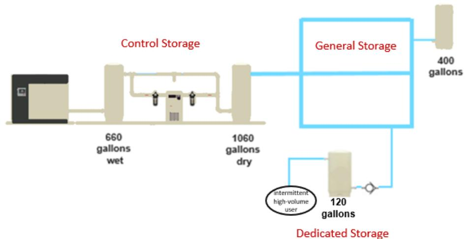
**Figure 4.21 Three types of storage in a compressed air system**
