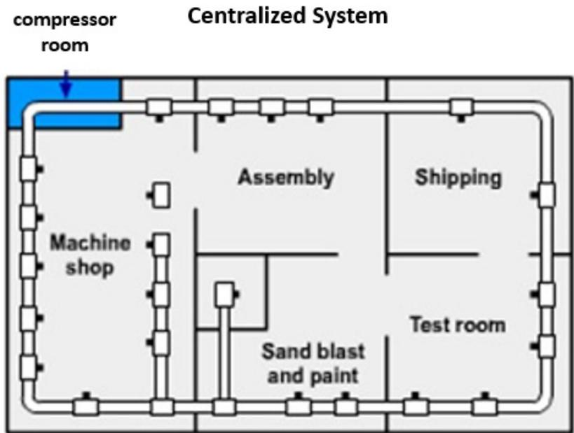
**Figure 4.15** Centralized system layout
