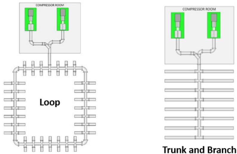
**Figure 4.17** Two basic distribution piping layouts
