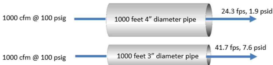
Figure 4.3 Pressure drop as a function of velocity.
