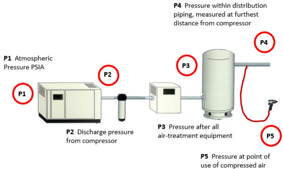
**Figure 4.5 Industry-accepted pressure naming convention used for compressed air systems**
