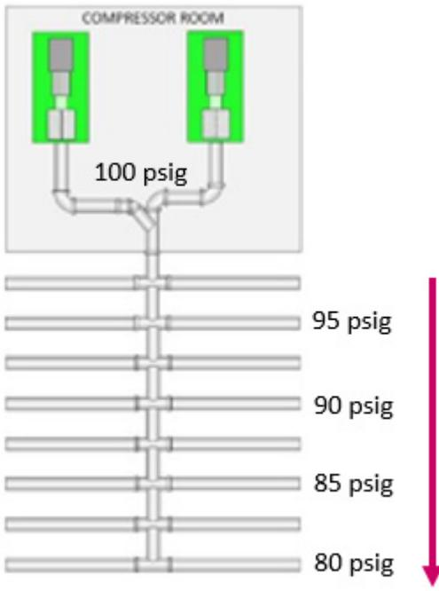
**Figure 4.18 Pressure drop in a trunk distribution layout**
