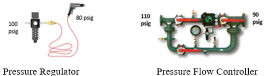
**Figure 4.7** Pressure regulation devices for managing artificial demand
