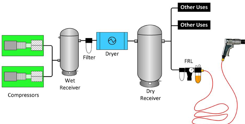
Figure 4.24 Wet and dry receivers as control storage
