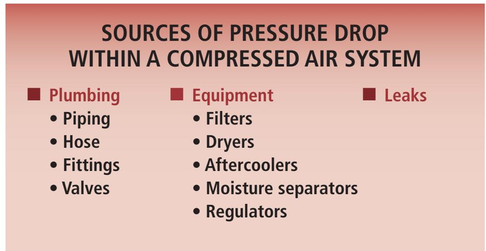
**Figure 4.4 Common sources of pressure drop**
