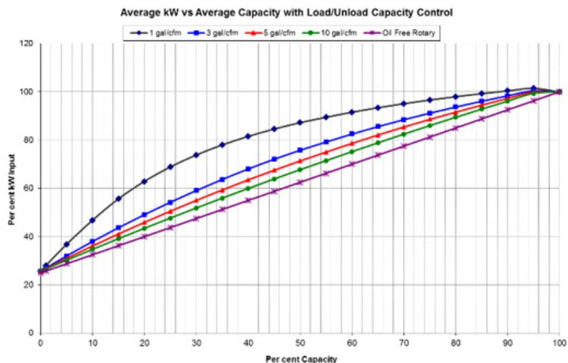
**Figure 4.23 Performance curve for a load/no load compressor as a function of control storage volume**
