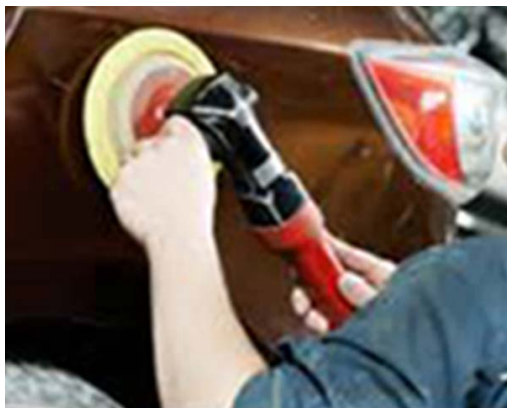
Figure 5.36: A polisher being used to put a final luster on an automobile.
