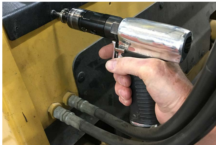
Figure 5.15: Pistol-grip screwdriver used in construction equipment assembly.
