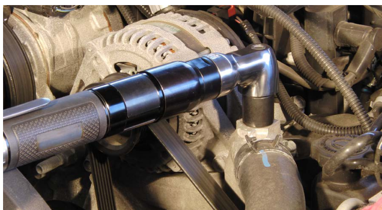
Figure 5.18: An angle nutsetter being used for automobile engine assembly.
