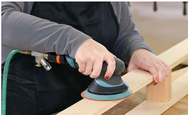
Figure 5.40: Random orbital sanders have a good operator control and provide a smooth, swirl-free finish.
