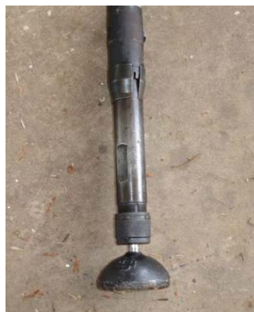
Figure 5.72: Backfill tamper with tamping pad.
