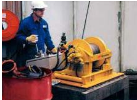
Figure 5.65: Utility hoist on the drill floor of an offshore drilling rig to handle drilling tools.
