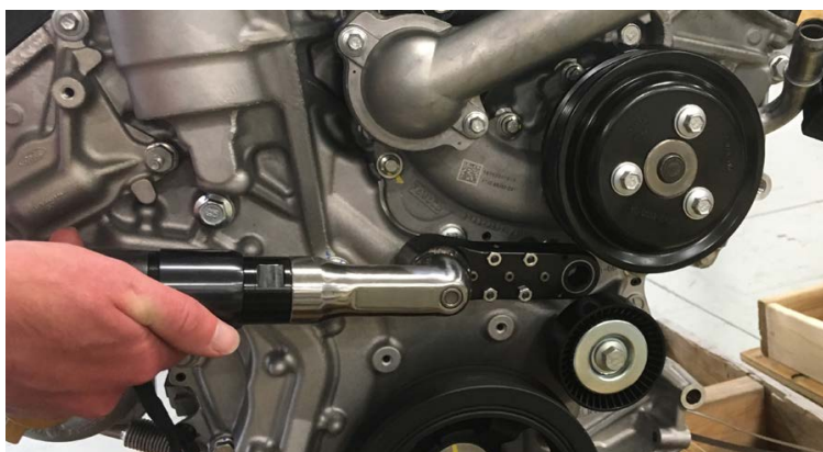
Figure 5.19: A crow-foot nutsetter is used where limited access to threaded fasteners precludes the use of other tool types.
