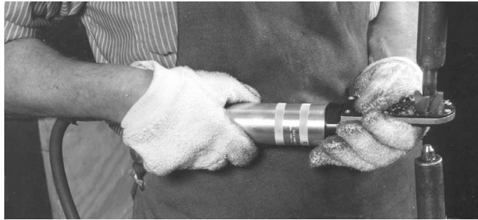
Figure 5.48: Electrode dressers quickly reshape electrodes to their original form for more effective welding.
