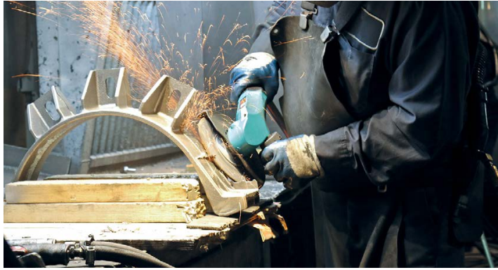
Figure 5.32: Right angle grinder being used to remove weld spatter from a fabricated part.
