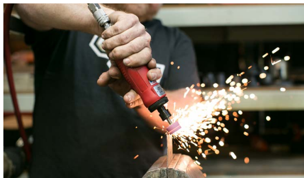
Figure 5.29: Die grinders are used for tool and die finishing, rapid removal of metal and burrs, and some weld finishing.
