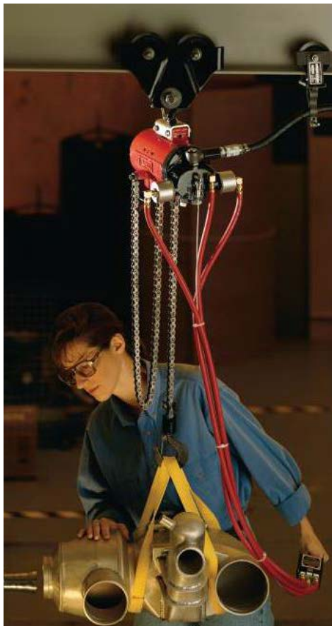
Figure 5.59: Air hoists are available with disc, drum or worm gear brakes.
