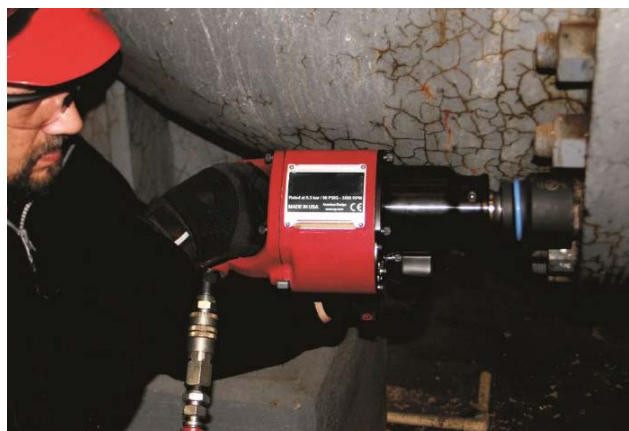
Figure 5.21: An impact wrench generates very high torque in a relatively small tool.
