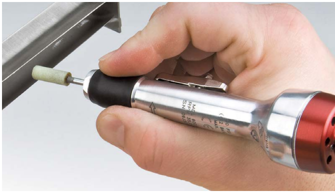
Figure 5.30: Turbine grinders are used for light metal removal where precision is important.
