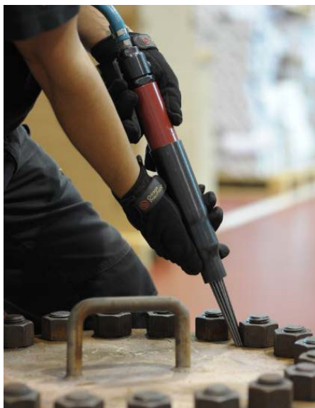
Figure 5.43: Needle scalers are well suited for cleaning weld flux, scale, paint and weld spatter.
