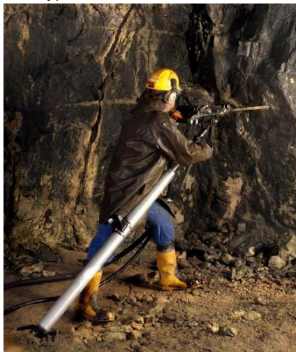
Figure 5.69: Stopper drill in use in a roof bolting operation.
