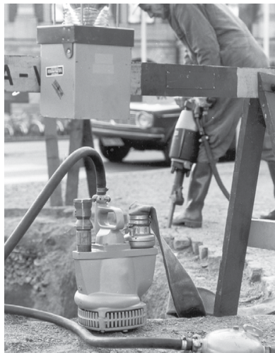
Figure 5.75: Centrifugal sump pump in use in construction application.
