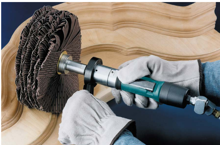
Figure 5.41: Sanding of double curved contours is made easy using a die grinder equipped with a flap wheel.
