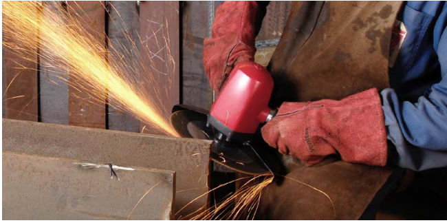
Figure 5.35: Vertical grinders are considered to be the most versatile and widely used of large-wheel grinders.
