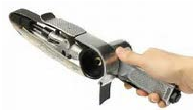
Figure 5.38: Belt sanders are used for fast removal of material, usually from wood parts.
