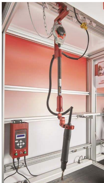
Figure 5.16: A balancer-suspended, straight style air screwdriver.
