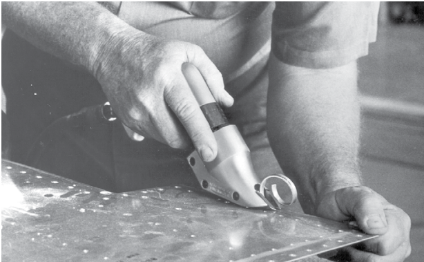
Figure 5.46: Air powered reciprocating shears are used to cut and trim sheet metal.
