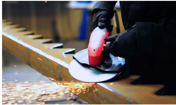
Figure 5.28: A wheel guard protects the operator from sparks and chips, and from wheel fragments if a wheel breaks.
