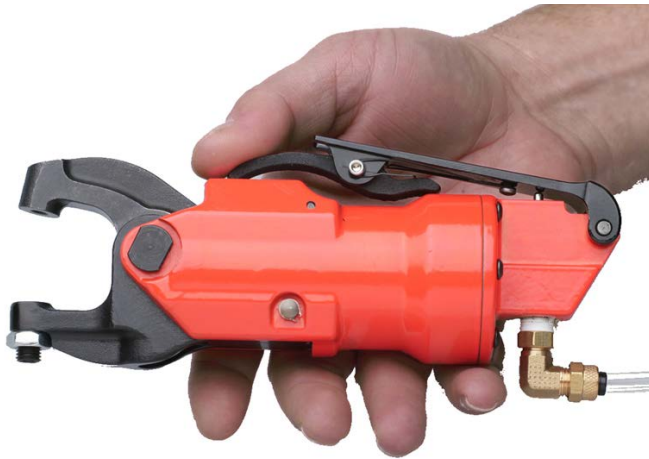
Figure 5.23: A compression riveter with a C-yoke that can be used to fasten a hinge to a metal frame.
