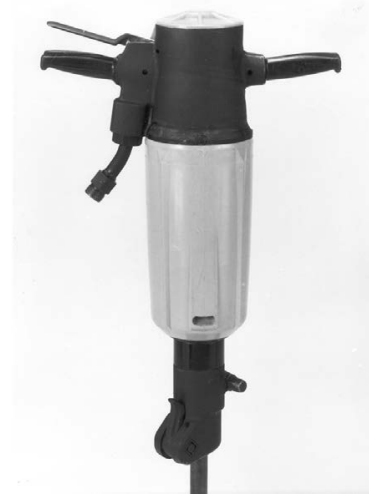
Figure 5.70: Silenced, vibration damped paving breaker.
