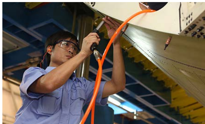
Figure 5.22: A riveting hammer for aircraft assembly.
