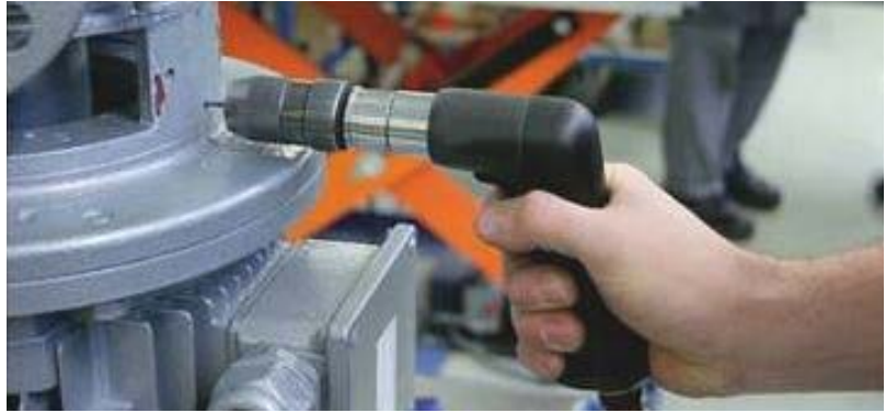
Figure 5.11: A portable air drill is used for drilling holes.
