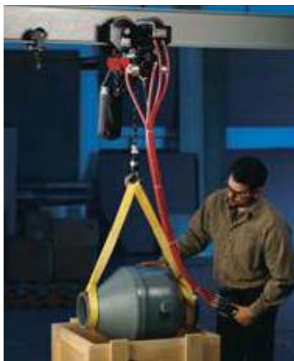
Figure 5.62: Power tractor-mounted hoist frees the operator from having to pull or push the load.
