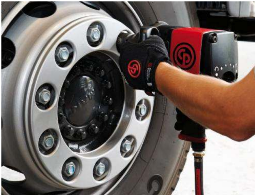
Pneumatic impact wrench installing tires.
