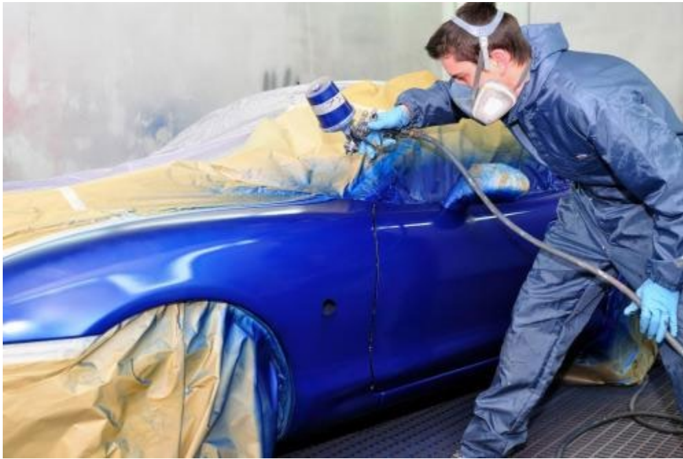
Paint for a car is applied using a compressed air powered sprayer.
